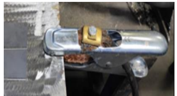
Proper clamped chassis
